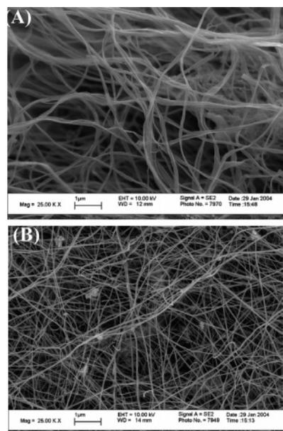
**Figure 1.** Structure of cellulose produced by two different *Acetobacter* strains clearly indicate differences. (A) NQ5, (B) E<sub>25</sub>; much larger cellulose ribbons of NQ5 are clearly distinguishable. Whereas the NQ5 strain creates a highly compact and rigid membrane, the E<sub>25</sub> strain produces a more gelatinous, yet still rigid form of cellulose, which is highly translucent (images captured by Dwight Romanovicz, University of Texas at Austin).
