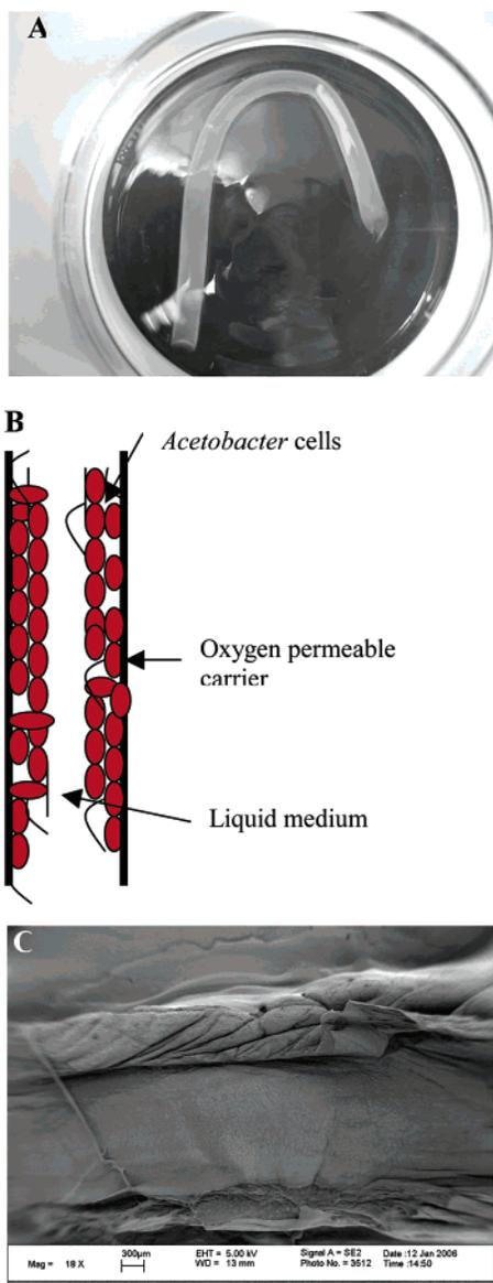
**Figure 3.** Hollow tube made from microbial cellulose according to the technique described by Roberts et al. (ref 64), using a silicon tube as a mold (A). *Acetobacter* cells which are highly aerobic organisms tend to gather in the oxygen-rich zones near the inner wall of the silicon tube where they produce and deposit cellulose (B). The inner surface (lumen) of the cellulose tube can be made very smooth and highly homogeneous (C).
